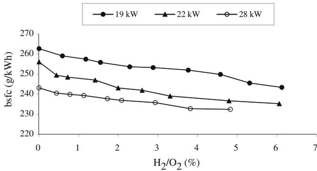
Fig. 4. Variation of brake specific fuel consumption (bsfc) with H<sub>2</sub>/O<sub>2</sub> percentage.
