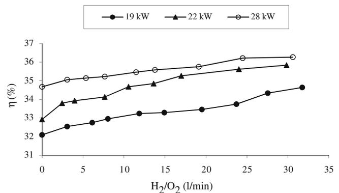
Fig. 3. Variation of brake thermal efficiency with H<sub>2</sub>/O<sub>2</sub> flow rate.
