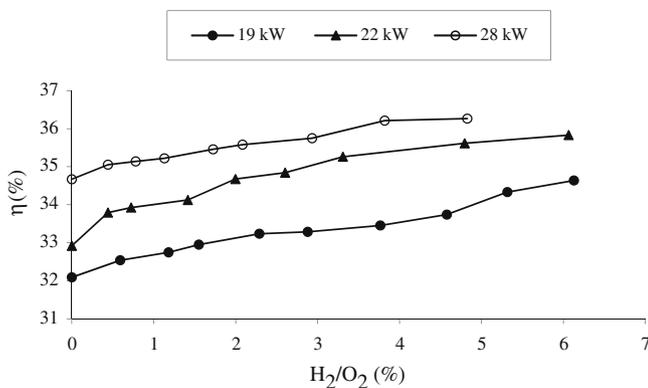
Fig. 2. Variation of brake thermal efficiency with H<sub>2</sub>/O<sub>2</sub> percentage.
