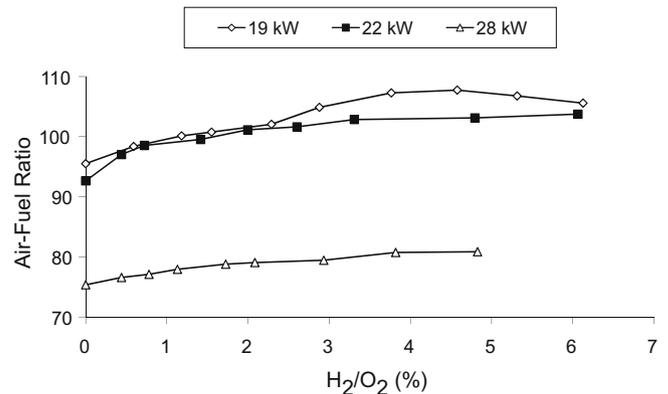
Fig. 7. Variation of air–fuel ratio with equivalent H<sub>2</sub>/O<sub>2</sub> percentage.
