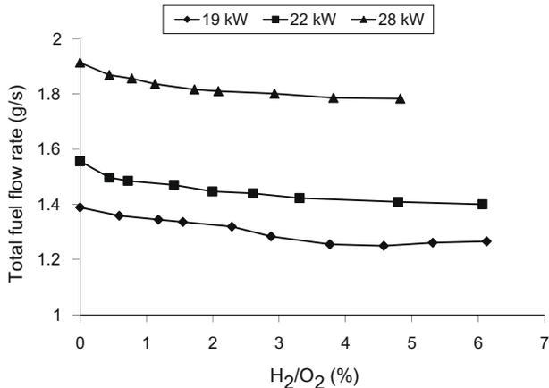
Fig. 5. Variation of total fuel flow rate with H<sub>2</sub>/O<sub>2</sub> percentage.
